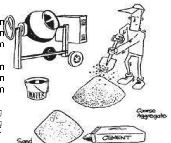
**Membuat 1 m3 beton mutu  $f'c = 9,8$  MPa (K 125), slump ( $12 \pm 2$ ) cm,  $w/c = 0,78$**
